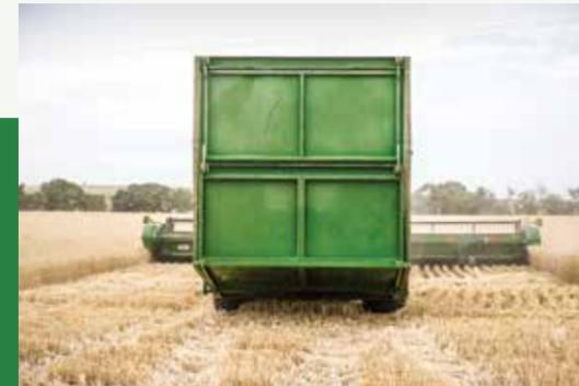
Large capacity 45m<sup>3</sup> on 3m tram lines
